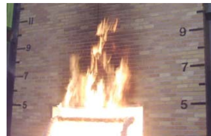
Figure 4: XPS Foam Insulation in Steel Stud Cavity Wall Mineral wool fire safing (min. 1" thick) is required in the header of all openings.
