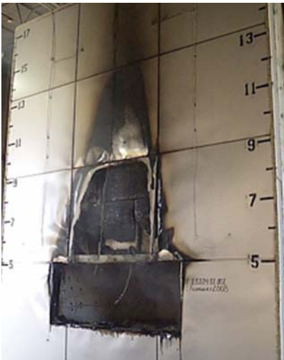
Figure 7: NFPA 285 Assembly Test With an NFPA 285 Approved Metal Composite Metal (MCM) Veneer and ASTM C1289 Type I Class 2 Fiberglass-Reinforced ISO Insulation (post-fire view)
