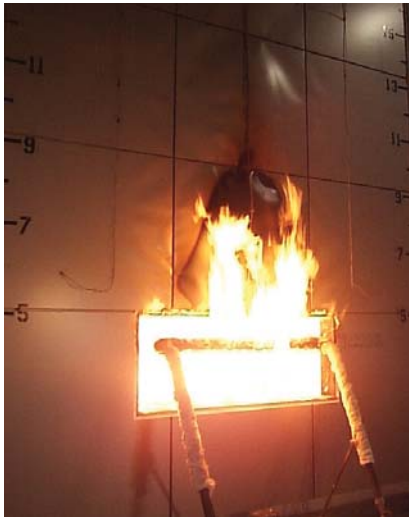
Figure 7: NFPA 285 Assembly Test With an NFPA 285 Approved Metal Composite Metal (MCM) Veneer and ASTM C1289 Type I Class 2 Fiberglass-Reinforced ISO Insulation (post-fire view)
