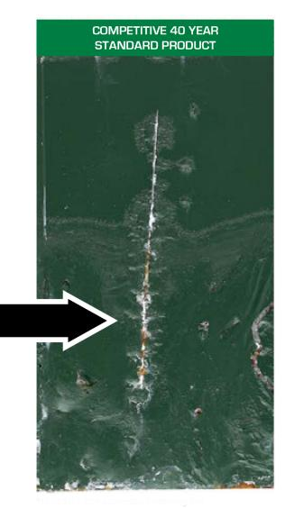
\* 2018 International Residential Code Table R905.10.3(2) Minimum Corrosion Resistance. Most states adopt the International Residential Code but there are exceptions. It's important to verify the state and local codes in your area to ensure compliance. \*\*ASTM B117-2016 Accelerated Weathering Test
