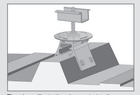
The above illustration demonstrates the RibBracket with the S-5-PV Kit attached.
