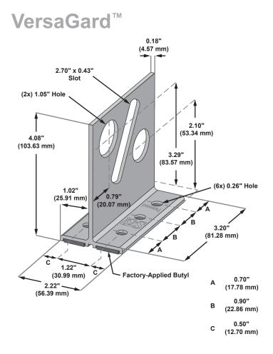
6 holes are provided for versatility. Some installations require only 2 fasteners. See the load table on the S-5! website and the installation instructions for more details.
